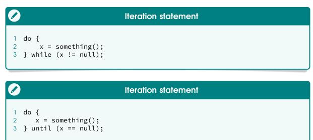
Finally, MVEL also implements the standard while, with the significant addition of an until counterpart (for inverted logic):
