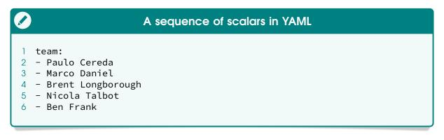
It is quite straightforward: team holds a sequence of four scalars. YAML also has flow styles, using explicit indicators rather than indentation to denote scope. The flow sequence is written as a comma-separated list within square brackets:
