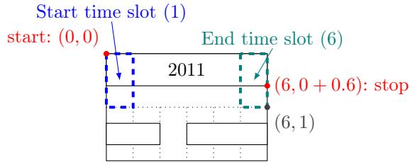
The figure below shows a Gantt chart with two lines and one (large) time slot and indicates the distances modified by these keys.
