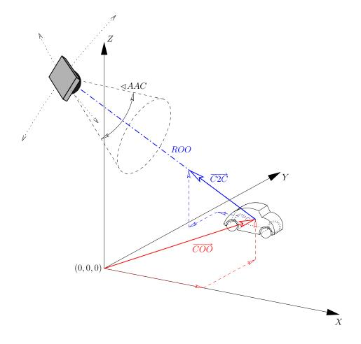
Figure 1: Camera and 3D object in the World System XYZ; centre of orbit position vector  $\vec{COO}$ , centre of orbit to camera direction vector  $\vec{C2C}$ , radius of orbit ROO, aperture angle of camera  $\triangleleft AAC$ .
