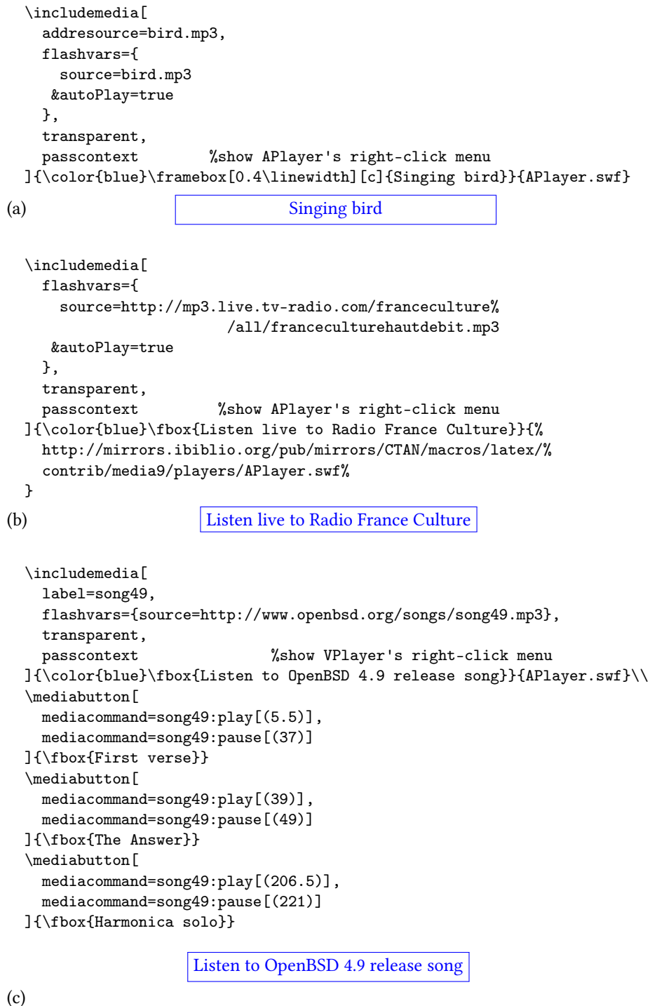
Figure 6: Example of (a) embedded sound file, (b) streamed audio and (c) progressively downloaded MP3. ID3 tags ‘title’, ‘artist’ and ‘album’ are displayed if contained in the MP3 stream or file. In (b), the sound player, APlayer.swf, is loaded from a CTAN mirror upon activation.
