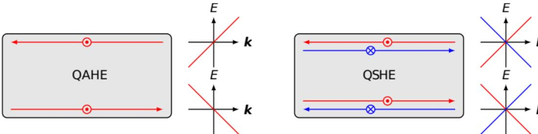
Conducting edge channels  $\longleftrightarrow$  Non-trivial bandstructure
