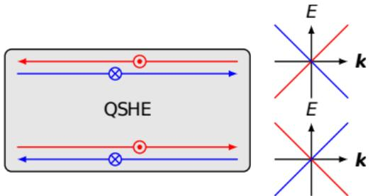
Conducting edge channels  $\longleftrightarrow$  Non-trivial bandstructure
