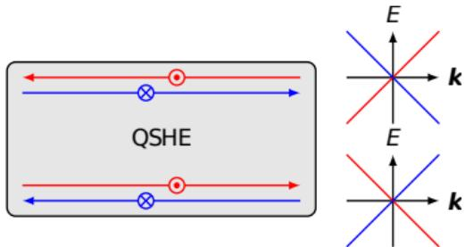
Conducting edge channels  $\longleftrightarrow$  Non-trivial bandstructure
