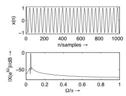
Figure 1: Sinusoid in time and frequency domain.
