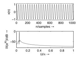
Figure 1: Sinusoid in time and frequency domain.
