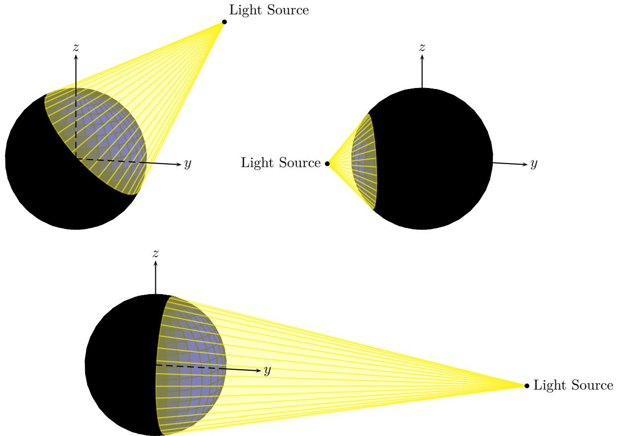
As you can see, the intersecting plane (section of the sphere with the cone of light) divides the object into two half spaces: the first half space (the one on the side of the light source) is illuminated and the other half space is the shadow region referring to this light source position.
