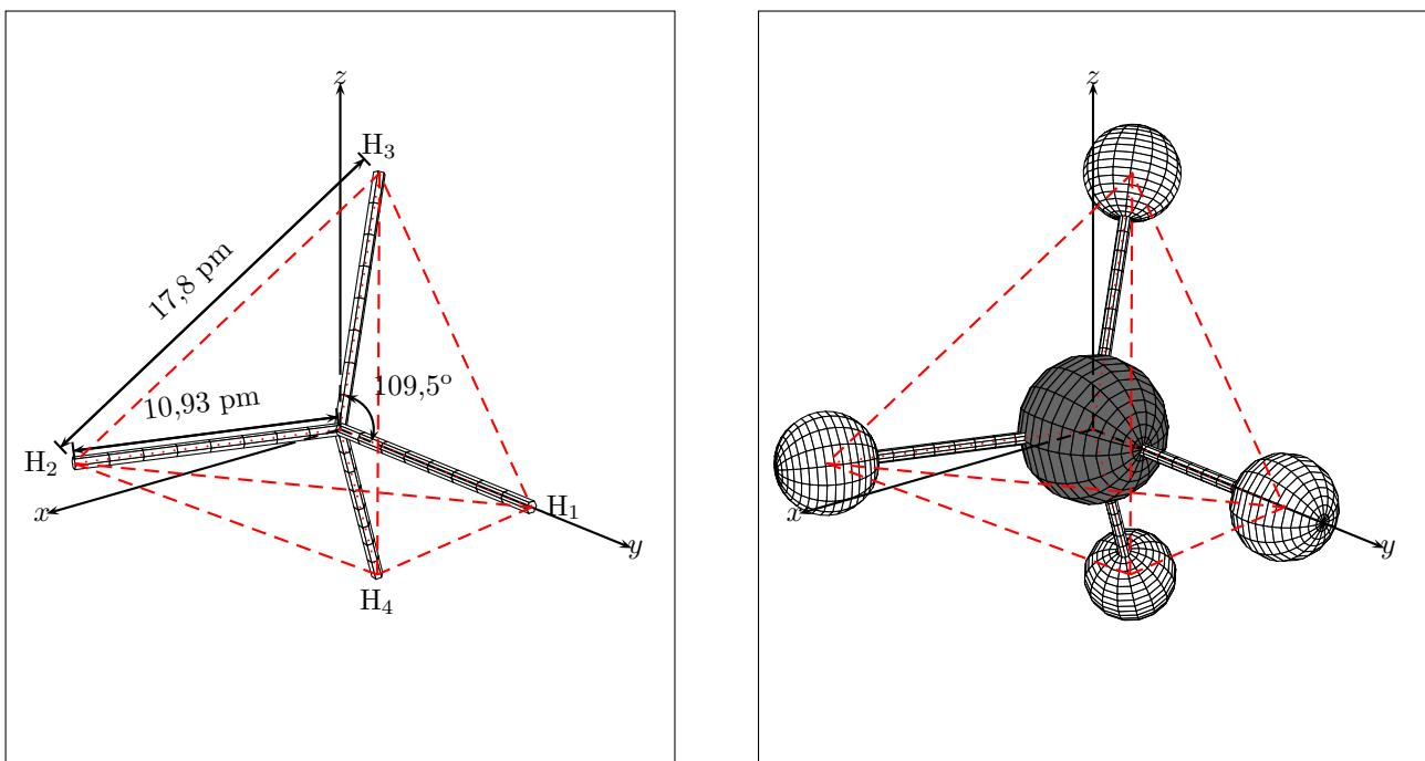
The construction of the molecule is detailed in the document `molecules.tex`. To add a dimensioning you only need to find the vertices of the tetrahedron:
