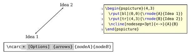
This connects the two nodes with an arc.
