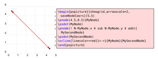
In the following example it doesn't work because the relative node setting via  $\protect\operatorname{rput}$  is not taken into account.
