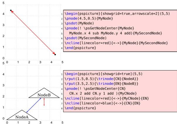
The coordinates of the nodes can also be saved with saveNodeCoors=true in global defined names N-<name>.x and N-<name>.y. With the optional argument NodeCoorPrefix, which is by default empty, the name setting can be changed to <NodeCoorPrefix><name>x and <NodeCoorPrefix><name>y.
