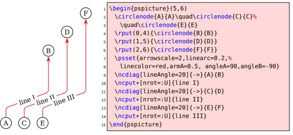
The \ncdiag macro sets the armB dynamically to the calculated value. Any user setting of armB is overwritten by the macro. The armA could be set to a zero length:
