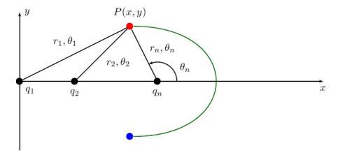
This problem possesses a cylindrical symmetry: it is thus sufficient to study the field and the potential in xy half-plane and the complete results are obtained by rotation around the x-axis.
