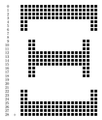
The width of the minimum bounding box for this character is 20; its height is 29. The '+' represents the reference pixel; notice how it lies outside the minimum bounding box. The *hoff* value is -2, and the *voff* is 28.
