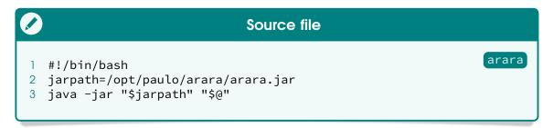
It is important to observe that the given full path must be properly quoted if it contains spaces. Note that the symbol used in the script body represents a special shell variable that stores all the actual parameters in a list of strings. This script file will act as the entry point for our tool. Now, we need to make it executable (i.e, set the corresponding execute permission) by running the following command in the terminal:
