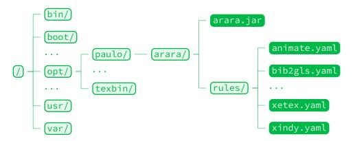
If the tool was built from source (as indicated in Section 8.2, on page 142), make sure to construct the provided directory structure previously presented. We can test the deployment by running the following command in the terminal (please note the full path):
