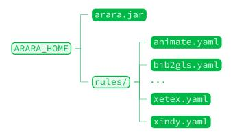
Provided that this specific directory structure is honoured, the tool is ready for use off the shelf. In fact, the official ororo package available in the release section of our project repository. Once the package is properly downloaded, we simply need to extract it into a proper ARARA\_HOME location.
