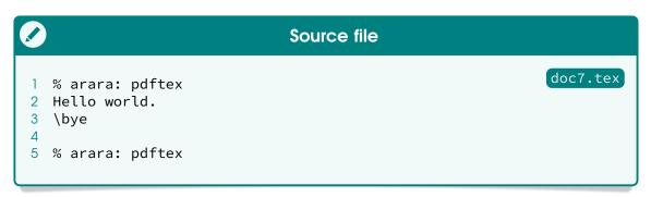
When running ororo without this option, two directives will be extracted (the ones found in lines 1 and 5). However, if executed with —header, the tool will only extract one directive (from line 1), as it will stop the extraction process as soon as it reaches line 2. This option can also be activated by default in the configuration file (see Section 4.2, on page 40).
