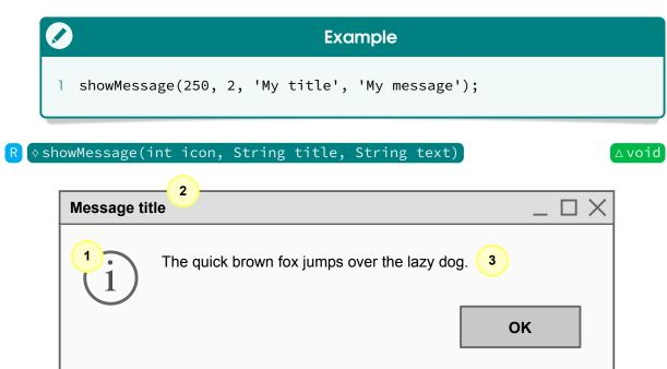
This method shows a message box according to the provided parameters. The dialog box is disposed when the user either presses the confirmation button or closes the window. It is important to observe that **ororo** temporarily interrupts the execution and waits for the dialog box disposal. Also note that the total time includes the idle period as well.
