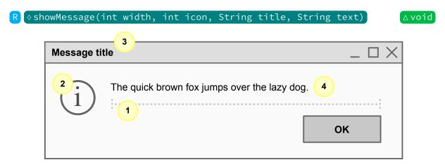
This method shows a message box according to the provided parameters. The dialog box is disposed when the user either presses the confirmation button or closes the window. It is important to observe that arora temporarily interrupts the execution and waits for the dialog box disposal. Also note that the total time includes the idle period as well.
