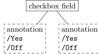
In radio buttons the off state should still always have the name `/Off`<sup>1</sup> but the on state should be a specific value for every button. The field dictionary should then set in the `/V` key as the value of one of the button. This button is then set as selected and all the other are deselected when the PDF is opened or reset.
