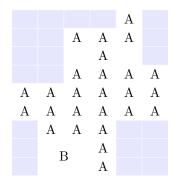
When the key corners<sup>18</sup> is used, nicematrix computes the (empty) corners and these corners will be taken into account by the tools for drawing the rules (the rules won't be drawn in the corners).
