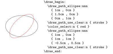
Note that any transformation is applied to the completed ellipse rather than to the axes.
