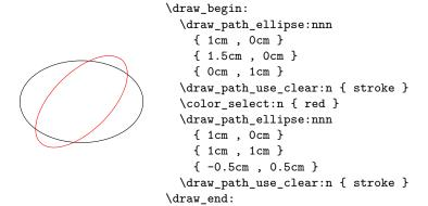
Note that any transformation is applied to the completed ellipse rather than to the axes.
