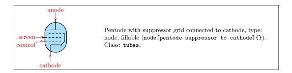
Note that the diodetube is used as component name to avoid clashes with the semiconductor diode. Normally, the filament is not drawn. If you want a filament, put the filament option in the node description:
