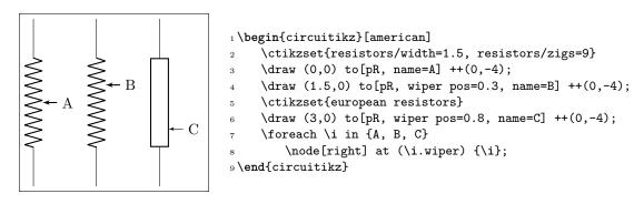
Since version 1.6.0, potentiometers and variable resistors have extra anchors<sup>12</sup>, to allow this kind of circuit (that seems to be common in some region):
