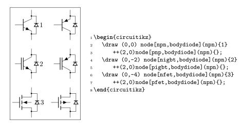
You can tweak the appearance of transistor's bodydiodes; see 4.15.8.
