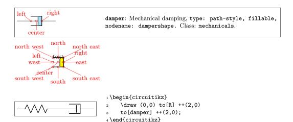
The command circuitdescbip\* is used to show the component description (you can check the definition and the usage looking at ctikzmanutils.sty file, and the \geolrcoord is used to show the main anchors (geographical plus left and right) of the component.
