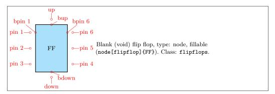
As you can see, in a void flip flop no external pins are drawn: you have to define the meaning of each of them to see them. To define a specific flip-flop, you have to set a series of keys under the \ctikzset directory multipoles/flipflop/, corresponding to pins 1...6, u for "up" and d for "down":
