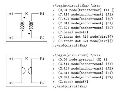
Moreover, you can access the two internal coils (inductances); if your transformer node is called T, they are named T-L1 and T-L2. Notice that the two inductors are rotated (by -90 degrees the first, +90 degrees the second) so you have to be careful with the anchors. Also, the midtap anchor of the inductors can be on the external or internal side depending on the numbers of coils. Finally, the anchors L1.a and L1.b are marking the start and end of the coils.
