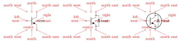
All transistors, except the multi-terminal bjtnpn and bjtpnp, (since 0.9.6) have internal nodes on the terminal corners, called inner up and inner down; you do not normally need them, but they are here for special applications:
