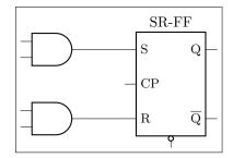
In this snippet, the coordinate (FF.pin 3 -| AND1.out) is the TikZ way to say "the point which is horizontally straight from FF.pin 3 and vertically form AND1.out". That way one can change the number -1 to move both AND ports nearer or farther away.
