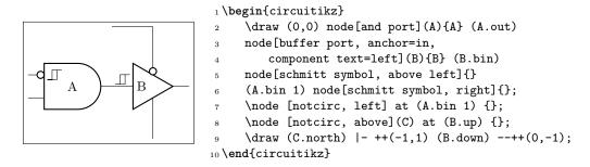
Notice the key component text=left that moves the label near to the left border of the component. There is also a \ctikzset{component text=left} if you prefer to have it as a default for all the IEEE ports.<sup>75</sup>
