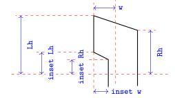
The default values are Lh = 8, Rh = 6, w = 3 and no inset: inset Lh = inset Rh = inset w = 0. In addition, you can set the following parameters:
