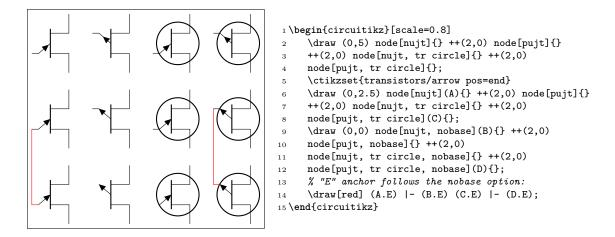
**4.15.5.10** Base/Gate terminal. The Base/Gate connection of all transistors can be disabled by the options *nogate* or *nobase*, respectively. The Base/Gate anchors are floating, but there is an additional anchor nogate/nobase, which can be used to point to the unconnected base:
