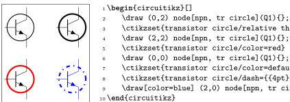
\ctikzset{transistor circle/relative thickness=2} \draw (2,2) node[npn, tr circle](Q1){}; \ctikzset{transistor circle/color=red} \draw (0,0) node[npn, tr circle](Q1){};
