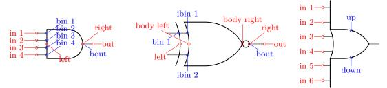
The inputs anchor are in *number* (on the tip of the lead) and bin *number* (border inputs) on the component's border (useful if you draw the ports with no inut leads). Additionally, you have ibin *number* (inner border inputs) for the x-type ports. The anchor named left is where a central border input would be.
