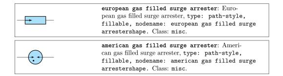
If (default behaviour) europeangfsurgearrester option is active (or the style [european gas filled surge arrester] is used), the shorthands gas filled surge arrester and gf surge arrester are equivalent to the european version of the component.
