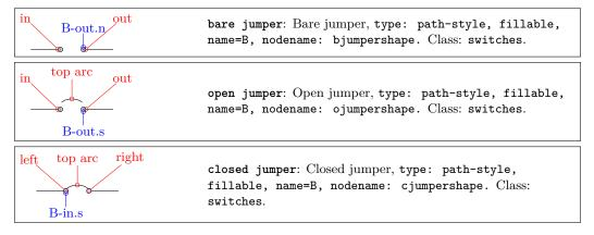
The top arc anchor can be used to locate the position of the top of the wire (when present). In bare jumper, the anchor is located in the middle of the connectors gap.
