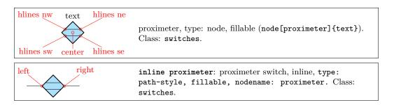
The proximeter shape<sup>72</sup> can be used as a dipole with the inline proximeter variant.
