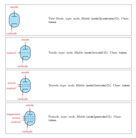
Some pentodes have the suppressor grid internally connected to the control grid, which saves a pin on the tube's housing.
