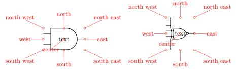
Most of the anchors can be seen in the following diagram:
