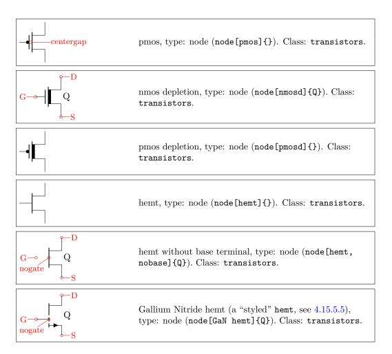
NFETS and PFETS have been incorporated based on code provided by Clemens Helfmeier and Theodor Borsche. Use the package options fetsolderdot/nofetsolderdot to enable/disable solderdot at some fet-transistors. Additionally, the solderdot option can be enabled/disabled for single transistors with the option solderdot and nosolderdot, respectively.
