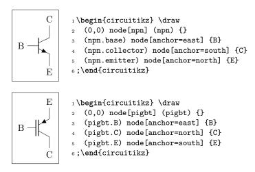
Notice that the geographical anchors of transistors are *not* affected by either the bodydiode and the circle options; the label text is also outside of them. This is to permit aligning the components independently from those features. On the other hand, this can sometimes create problems because that element is outside the bounding box automatically calculated by TikZ.
