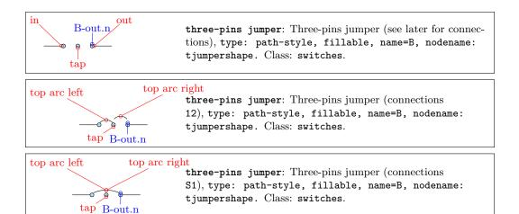
The option is used as shown in the following example, or by setting the key using  $\texttt{\ctikzset}$ . The value must be two characters, either two numbers (where 0 means "bare", 1 means "open", and 2 means "closed") or the letter S (for "span") and one number. In the latter case, the arc will connect the fist and last pole<sup>73</sup>
