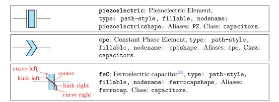
Capacitors are fillable since v1.4.1; this is normally just a stylistic option but in the case of ferroelectric capacitors that could be used to show the state of the hysteresis of the component.
