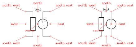
The other anchors behave similarly to the transistor's ones; you also have access to the internal components nodes by using <code>nodename-R</code> and <code>nodename-L</code> names for the right and left element, which is supposed to be <code>T</code> in the drawing below. Be wary that given that here you can (see later) reverse the direction of one or both of the elements, the rotation (and so the anchors) is not fixed (you can see that in the blue and green examples below).
