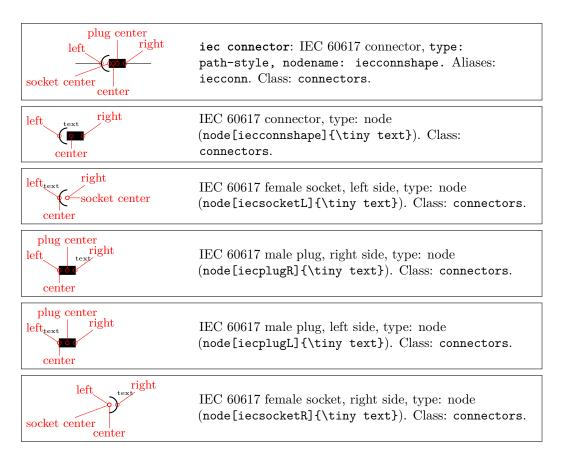
The center anchors (as well as the text position) of the split elements of the connectors are on the side of the component (similar to what happens with grounds and supply voltage arrows) to ease the most common use.
