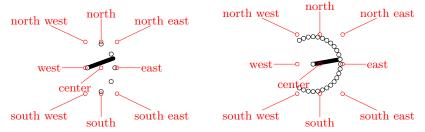
In addition to the anchors they have in common with the cute switches, the rotary switch has the so called "angled" anchors and the "external square anchors". *Angled anchors*, called aout 1, aout 2 and so forth, are anchors placed on the output poles at the same angle as the imaginary lines coming from the input pole; *square anchors*, called sqout 1..., are located on an imaginary square surrounding the rotary switch on the same line.
