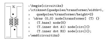
Transformers also inherit the inductors/scale (see 4.3.5) and similar parameters. It's your responsibility to set the aforementioned parameters if you change the scale or width of inductors.
