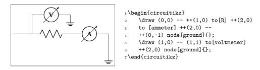
Since version 0.9.0 you have more options for the measuring instruments. You can use the generic rmeterwa (round meter with arrow), to which you can specify the internal symbol with the option t=... (and is fillable).
