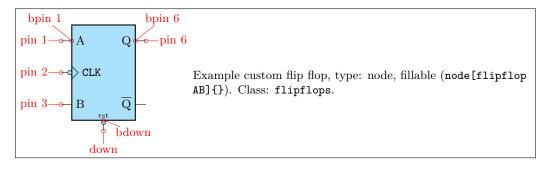
RST (created by RST). By default, the following flip-flops are defined, as well as a support shape for the clock wedge:
