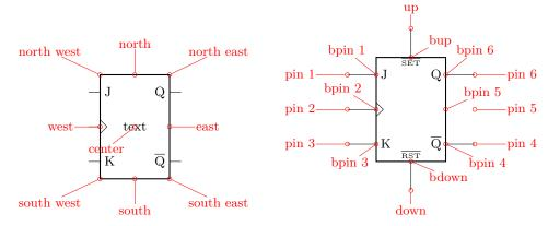
If you have negated pins, you can access the ocirc shapes with the name as <nodename>-N<pin number>, and all the respective anchors (for example — myFFnode-N4.west).
