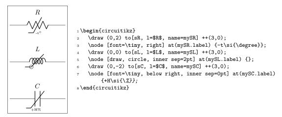
The anchor is positioned just on the corner of the segmented line crossing the component.
