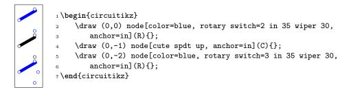
**4.21.4.2** Rotary switch customization Apart from the basic customization seen above (number of channels, etc.) you can change, as in the cute switches, the shape used by the connection points with the parameter multipoles/rotary/shape, and the thickness of the wiper with multipoles/rotary/thickness. The optional arrow has thickness equal to the standard bipole thickness bipoles/thickness (default 2).
