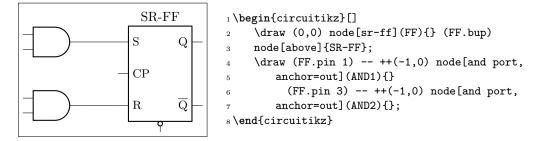
You can notice a pair of things here: first of all, the use of the **anchor=out** in the port, to tell TikZ that we want the node moved so that the **out** anchor is the reference one. The second one is that we have repeated the absolute shift (the ++(-1, 0)) twice. This is a bad practice; it is much better to have the "free" parameters of a schematic just stated once, so that we can change them in just one point.
