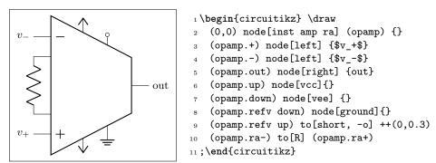
Amplifiers also have "border" anchors (just add b, without space, to the anchor, like b+ or bin up and so on). These can be useful to add "internal components" or to modify the component. Also the leftedge anchor (on the border midway between input) is available.
