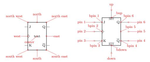
If you have negated pins, you can access the ocirc shapes with the name as <nodename>-N<pin number>, and all the respective anchors (for example — myFFnode-N4.west).
