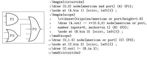
As you can see, the **center** anchor is (for historic reasons) not in the center at all. You can fix this with the command **\ctikzset{logic ports origin=center}**:
