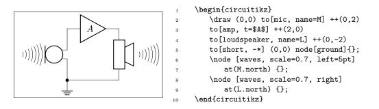
You have two types of microphones; mic has protruding connection and tlmic (for tail-less microphone) is inline. This last one is handy for use as a separate shape (which is named tlmicshape). You can change the (relative) thickness of the straight bar using the key bipoles/mic/bar thickness (default 1).
