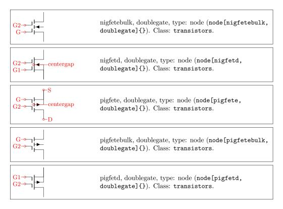
You can use the double-gated transistor for example like this:<sup>50</sup>
