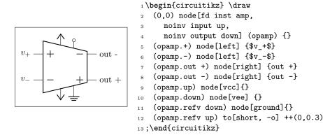
When you use the noinv input/output  $\ldots$  keys the anchors (+, -, out +, out -) will change with the effective position of the terminals. You also have the anchors in up, in down, out up, out down that will not change with the positive or negative sign.
