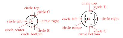
The multi-terminal transistors have all the geographical anchors; note though that the **center** anchor is not the geometrical center of the component, but the logical one (at the same height as the base). The additional anchors **vcenter** (vertical geometric center of the collector-emitter zone) and **gcenter** (graphical center) are provided, as shown in the following picture. They have no bodydiode anchors nor **inner** *up/down* ones.
