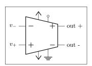
1 \begin{circuitikz} \draw 2 (0,0) node[fd inst amp] (opamp) {} (opamp.+) node[left] {\$v\_+\$} 3 (opamp.-) node[left] {\$v\_-\$} 4 (opamp.out +) node[right] {out +} 5 (opamp.out -) node[right] {out -} 6 (opamp.up) node[vcc]{} 7 (opamp.down) node[vee] {} 8 (opamp.refv down) node[ground]{} 9 (opamp.refv up) to[short, -o] ++(0,0.3)10 11;\end{circuitikz}
