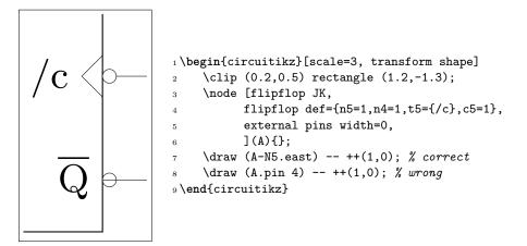
Normally the symbols on the flip-flop are un-rotated when you rotate the symbol, but as in case of chips, you can avoid it.
