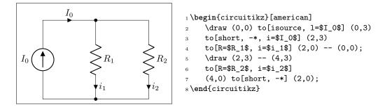
One of the problems with this circuit is that we would like to have the current labels in a different position, such as for example on the upper side of the resistors, so that Kirchoff's Current Law at the node is better shown to students. No problem; as you can see in section 5.2 you can use the position specifiers <>^\_ after the key i:
