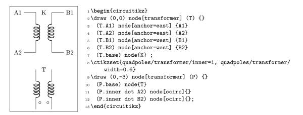
This can be useful if you want to put seamlessly something in series with either side of the component; for simplicity, you have a style setting quadpoles style to toggle between the standard shape of double bipoles (called inward, default) and the one without horizontal leads (called inline):
