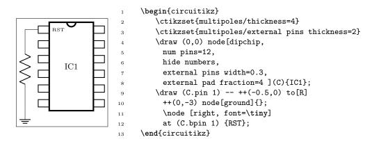
Also, you can suppress the drawing of the pins, by using the style no inputs leads (that can be reverted with input leads). The main difference between setting external pins width to 0 or using no inputs lead is that in the first case the normal pin anchors and the border anchors will coincide, and in the second case they will not move and stay where they should have been if the leads were drawn.
