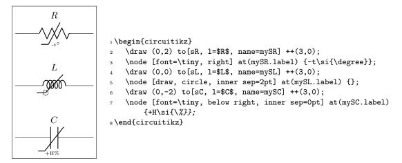
The anchor is positioned just on the corner of the segmented line crossing the component.
