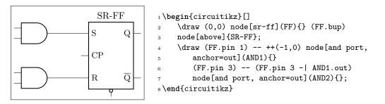
In this snippet, the coordinate (FF.pin 3 - | AND1.out) is the TikZ way to say "the point which is horizontally straight from FF.pin 3 and vertically form AND1.out". That way one can change the number -1 to move both AND ports nearer or farther away.
