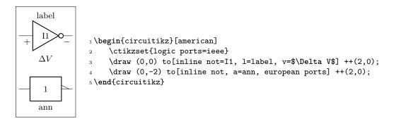
Notice that in the inline version the leading pins are not drawn, so in the case of the transmission gates you have to use the border pins to connect the gates.
