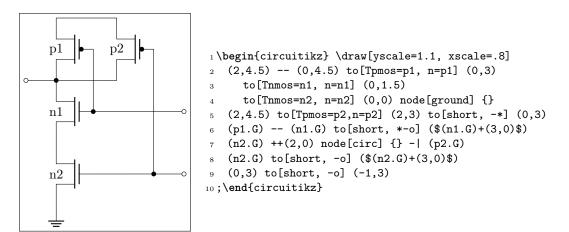
Transistors used in path are fully path-style components, so to flip and rotate them you should use mirror and invert as shown in section 3.1.4.2.
