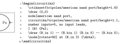
In an analogous manner, there is a setting logic ports draw output leads (and a corresponding style no output leads) that suppresses the drawing of the output lead. A shortcut boolean key logic ports draw leads will suppress or enable all leads (the corresponding styles are no leads and all leads).
