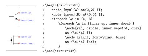
Additionally, you can access the position for the flyback diodes and possibly snubbers as shown in 4.15.5.4.
