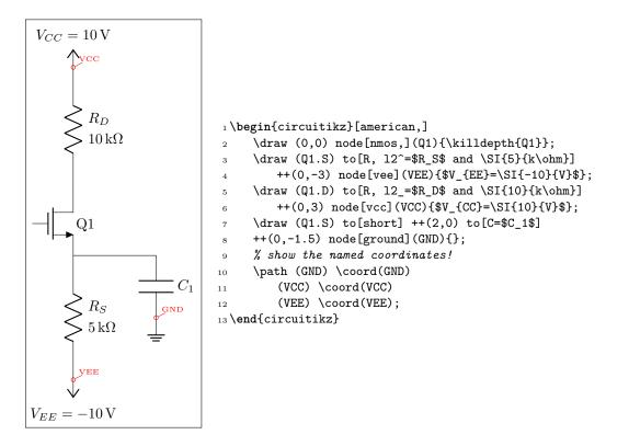
After that, let's add the input part. I will use a named node here, referring to it to add the input source. Notice how the ground node is positioned: the coordinate (in |- GND) is the point with the horizontal coordinate of (in) and the vertical one of (GND), lining it up with the ground of the capacitor  $C_1$  (you can think it as "the point aligned vertically with in and horizontally with GND").
