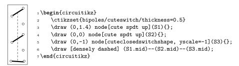
Finally, the switches are normally drawn using the ocirc shape, but you can change it, as in the following example, with the key bipoles/cuteswitch/shape. Be careful that the shape is used with its defaults (which can lead to strange results), and that the standard anchors will be correct only for circ and ocirc shapes, so you have to use the internal node syntax to connect it.
