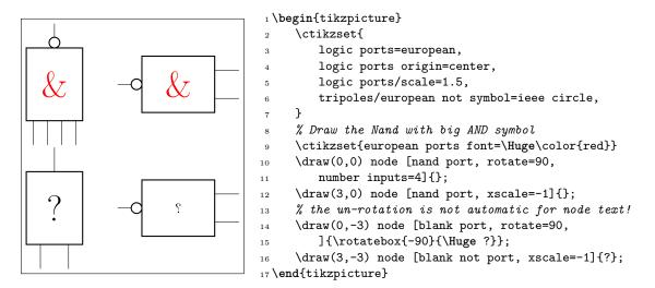
**4.22.7.1 European logic port customization** Normally the European-style logic port with inverted output are marked with a small triangle; if you want you can change it with the key tripoles/european not symbol; its default is triangle but you can set it to circle like in the following example. As you can see, the circle size is the same as the circuit poles; if you prefer the size used in the IEEE standard ports, you can use set it to ieee circle.
