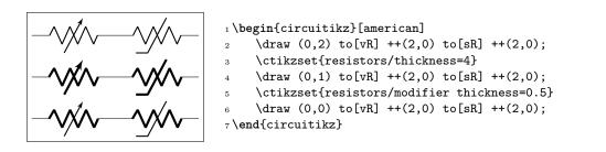
**4.2.3.3 Arrows.** You can change the arrow tips used in tunable resistors (vR, tgeneric) with the key tunable end arrow and in potentiometers with the key wiper end arrow (by default the key is the word "default" to obtain the default arrow, which is latexslim for both). Also you can change the start arrow with the corresponding tunable start arrow or wiper start arrow (the default value "default" is equivalent to {} for both, which means no arrow).
