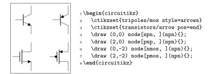
If the option arrowmos is used (or after the command \ctikzset{tripoles/mos style/arrows} is given), this is the output:
