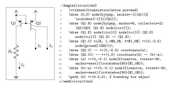
Here is one composite example (please notice that the xscale=-1 style would also reflect the label of the transistors, so here a new node is added and its text is used, instead of that of pnp1):
