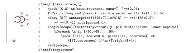
A similar approach can be used for dependent sources. Just remember that the anchors move (rotate) together with the component.
