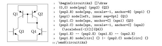
Notice that the text labels of transistors are outside the bounding box of the component (that is, the set of geographical anchors). If it is a problem, use a separate text node to set the transistor's label. Of course, transistors like other components can be reflected vertically:
