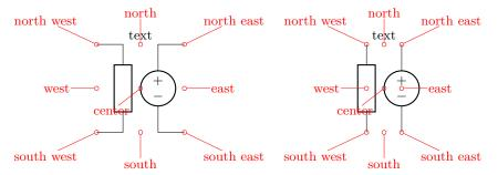
The other anchors behave similarly to the transistor's ones; you also have access to the internal components nodes by using *nodename*-R and *nodename*-L names for the right and left element, which is supposed to be T in the drawing below. Be wary that given that here you can (see later) reverse the direction of one or both of the elements, the rotation (and so the anchors) is not fixed (you can see that in the blue and green examples below).
