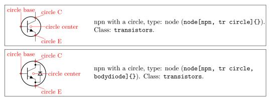
The position of the circle on collector and emitter by default is the one shown above; the position along the base can be adjusted in most transistors using the \ctikzset parameter transistor circle/default base in (by default 0.9); njfet and pjfet use transistor circle/njfet
