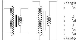
You can obviously define a style for a "non-standard" transformer. For example, you can have a current transformer<sup>73</sup> defined like this:
