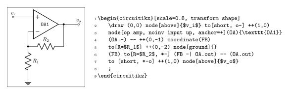
The last step to obtain the final look is to add a bit of styling. We want the op-amp filled with a light cyan color, and we prefer to have the label aligned with the left side of the device:
