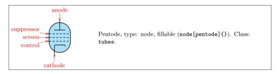
Some pentodes have the suppressor grid internally connected to the control grid, which saves a pin on the tube's housing.
