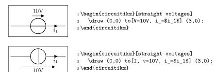
And you can override that with **bipole/is voltage** keeping into account that the default direction will be the one of passive components (see 5.2.2):
