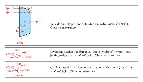
You can define a custom shape for the muxdemuxes using an interface similar to the one used in flip-flops; for example:
