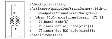
Transformers also inherit the inductors/scale (see 4.3.5) and similar parameters. It's your responsibility to set the aforementioned parameters if you change the scale or width of inductors.
