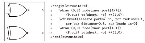
In addition to the specific parameters, you can also apply to these ports the boolean style **no input leads** as in legacy ones (this simply *does not draw* the input leads, but the anchors stays where they should):
