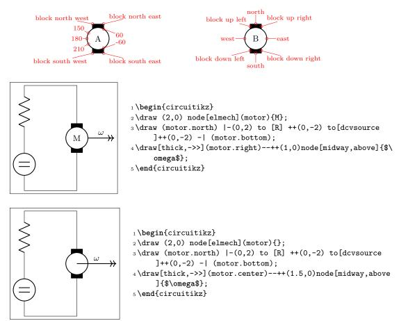
The symbols can also be used along a path, using the transistor-path-syntax(T in front of the shape name, see section 4.15.10). Don't forget to use parameter n to name the node and get access to the anchors:
