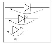
The value of distance from node can also be an absolute distance; in that case is measured from the start of the connection toward the component on the left (and symmetrically on the right), so this will put the start and end point to 0.25 cm from the start of the node:
