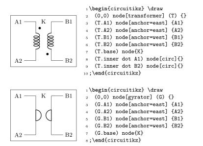
Moreover, you can access the two internal coils (inductances); if your transformer node is called T, they are named T-L1 and T-L2. Notice that the two inductors are rotated (by -90 degrees the first, +90 degrees the second) so you have to be careful with the anchors. Also, the midtap anchor of the inductors can be on the external or internal side depending on the numbers of coils. Finally, the anchors L1.a and L1.b are marking the start and end of the coils.
