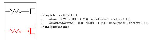
You can change this behavior by setting the key tripoles/nmosd/depletion color (default value default, which means "use the draw color") to the color you want; using none will lead to an unfilled channel (note that in this case the color does not change automatically with the path!):
