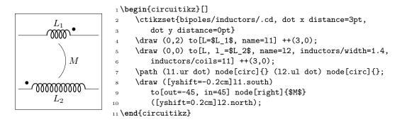
Notice that the position of the dot anchors does not coincide with the position of the dots in the transformers (see section 4.19), because there they depend on the size of the complete double-bipole more that on the size of the inductances.
