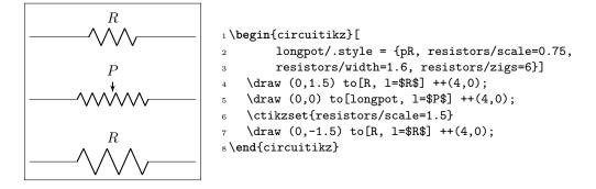
**4.2.3.2** Thickness. The line thickness of the resistive components is governed by the class thickness; you can change it assigning a value to the key resistors/thickness (default none, that means bipoles/thickness is used, and that defaults to 2.0; the value is relative to the base line thickness).
