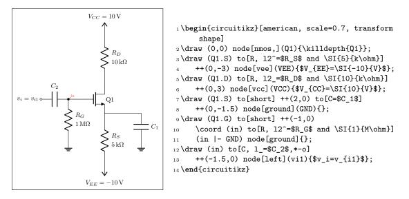
Notice that the only absolute coordinate here is the first one, (0,0); so the elements are connected with relative movements and can be moved by just changing one number (for example, changing the to[C=\$C\_1\$] ++(0,-1.5) will move *all* the grounds down).
