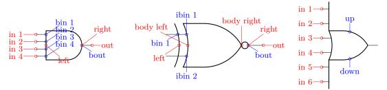
The inputs anchor are in *number* (on the tip of the lead) and bin *number* (border inputs) on the component's border (useful if you draw the ports with no inut leads). Additionally, you have ibin *number* (inner border inputs) for the *x*-type ports. The anchor named left is where a central border input would be.
