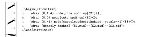
**4.21.2.2** Cute switches customization You can use the key bipoles/cuteswitch/thickness to decide the thickness of the switch lever. The units are the diameter of the ocirc connector, and the default is 1.
