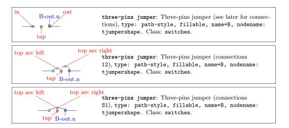
The option is used as shown in the following example, or by setting the key using <code>\ctikzset</code>. The value **must** be two characters, either two numbers (where 0 means "bare", 1 means "open", and 2 means "closed") or the letter S (for "span") and one number. In the latter case, the arc will connect the fist and last pole<sup>80</sup>
