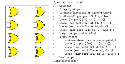
**4.22.5.1** American logic port customization Logic port class is called logic ports, so you can scale them all with logic ports/scale (default 1.0).
