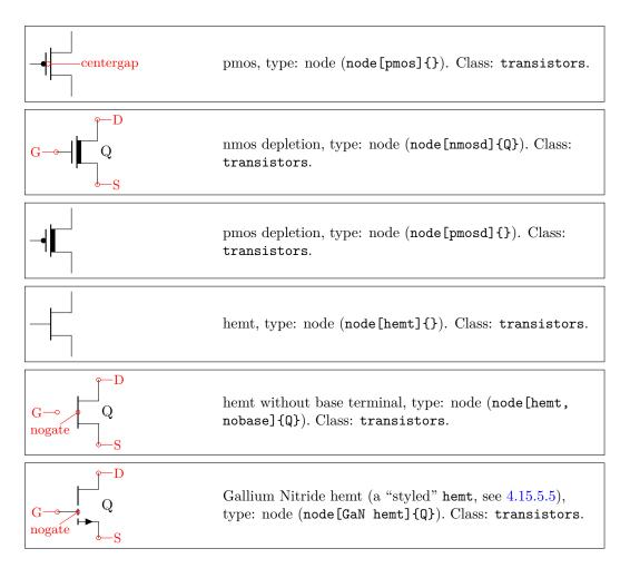
NFETS and PFETS have been incorporated based on code provided by Clemens Helfmeier and Theodor Borsche. Use the package options fetsolderdot/nofetsolderdot to enable/disable solderdot at some fet-transistors. Additionally, the solderdot option can be enabled/disabled for single transistors with the option solderdot and nosolderdot, respectively (You can adjust the size of the solder dot, see section 4.15.5.12).
