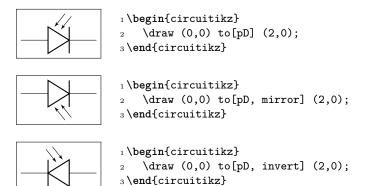
Placing labels, currents and voltages also works, please note, that mirroring and inverting does not influence the positioning of labels and voltages. Labels are by default above/right of the bipole and voltages below/left, respectively.
