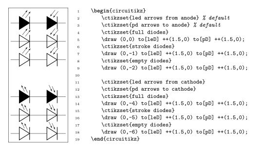
Since version  $1.5.5^{21}$ , you can change the arrows used for LEDs, photodiodes and laser diodes with the generic arrows options shown in 4.2.3.3, using the name opto, like in the following (overdone) example. Normally you want just to change the end arrow...
