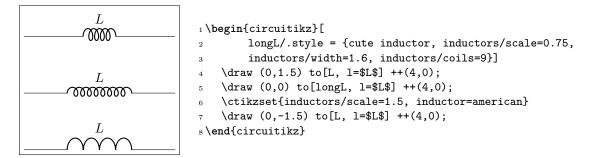
**4.3.5.1** Chokes can have single and double lines, and can have the line thickness adjusted (the value is relative to the thickness of the inductor). In general, you should use the anchors (see 4.3.6.2) to add core lines to inductors.
