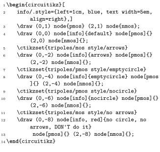
You can also change<sup>54</sup> the type of the arrow for the "light rays" of the phototransistors with the generic arrows options shown in 4.2.3.3, using the name opto, like in the following (overdone) example. Also the opto arrows styling options (see section 4.4.3.1).
