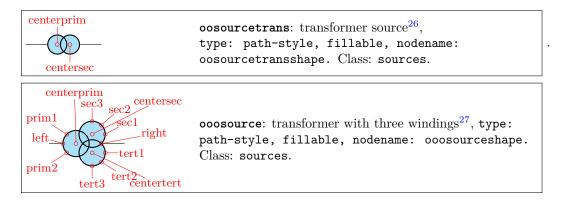
The transformer shapes vector group options can be specified for the primary (prim=value), the secondary (sec=value) and tertiary (tert=value) three-phase vector groups: the value can be one of delta, wye, eyw<sup>28</sup> and zig.
