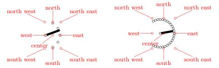
In addition to the anchors they have in common with the cute switches, the rotary switch has the so called "angled" anchors and the "external square anchors". Angled anchors, called **aout 1**, **aout 2** and so forth, are anchors placed on the output poles at the same angle as the imaginary lines coming from the input pole; square anchors, called **squut 1**..., are located on an imaginary square surrounding the rotary switch on the same line.
