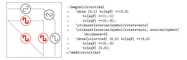
**4.5.9.3** Polarity symbols. The symbols drawn into the american voltage source<sup>31</sup> can be changed by using the \ctikzset keys bipoles/vsourceam/inner plus and .../inner minus (by default they are \$+\$ and \$\vphantom{+}-\$ respectively, in the current font), and move them nearer of farther away by twiddling bipoles/vsourceam/margin (default 0.7, less means nearer). The reason of the \vphantom can be found in section 5.5.6.
