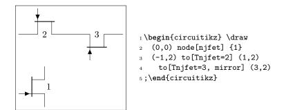
Access to the gate and/or base nodes can be gained by naming the transistors with the **n** or **name** path style:
