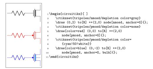
Obviously you have the equivalent tripoles/pmosd/depletion color for type-P transistors. They also have path-style syntax, as the other transistors.
