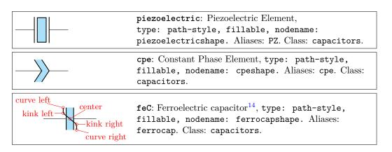
Capacitors are fillable since v1.4.1; this is normally just a stylistic option but in the case of ferroelectric capacitors that could be used to show the state of the hysteresis of the component.
