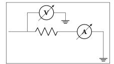
Since version 0.9.0 you have more options for the measuring instruments. You can use the generic rmeterwa (round meter with arrow), to which you can specify the internal symbol with the option t=... (and is fillable).
