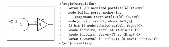
Notice the key component text=left that moves the label near to the left border of the component. There is also a \ctikzset{component text=left} if you prefer to have it as a default for all the IEEE ports.<sup>82</sup>
