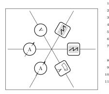
\begin{circuitikz}[scale=0.8, transform shape] 1 \ctikzset{rotated instruments} % new default  $\mathbf{2}$ \draw (0,0) to[oscope] ++(0:3); 3 \draw (0,0) to[oscope] ++(60:3); 4 \draw (0,0) to[rmeter, t=A] ++(120:3);  $\mathbf{5}$ % local override 6 \draw (0,0) to[rmeterwa, t=A, straight instruments] 7 ++(180:3); \ctikzset{straight instruments} % back to default 8 \draw (0,0) to[rmeterwa, t=A] ++(240:3); 9 % local override 10 \draw (0,0) to[smeter, t=A, rotated instruments] ++(300:3);
